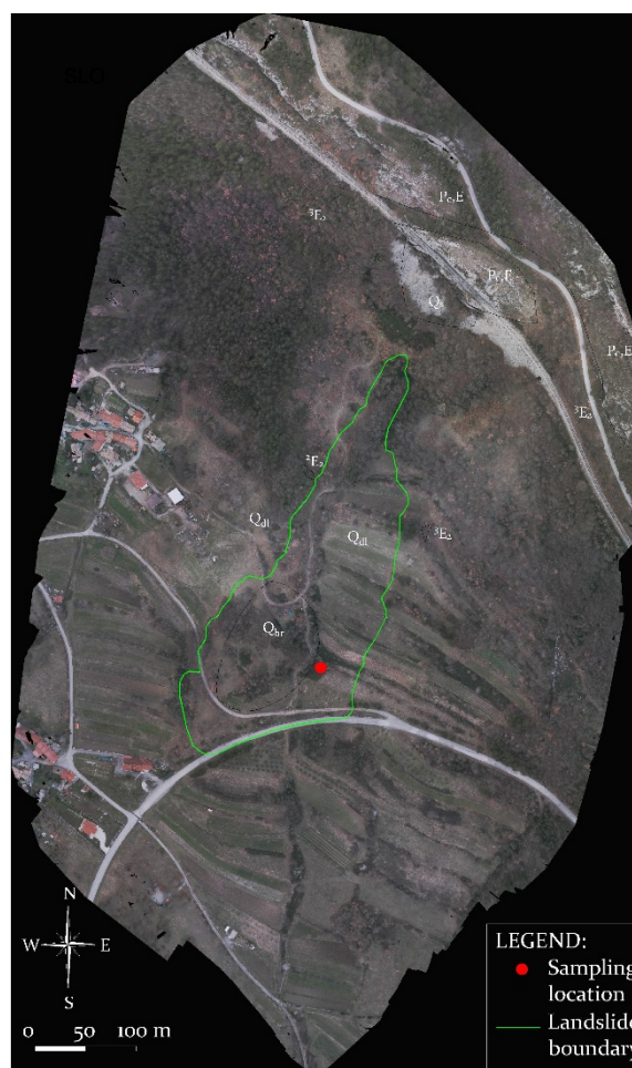
Figure 1 Krbavčići landslide on a detailed orthophoto map from 2016 with sampling location and landslide boundary ( Q_{(br,dl)} -cover deposits, {}^3(2)E_2 -marl and siltstone outcrops, P_{c,E} -limestone).
