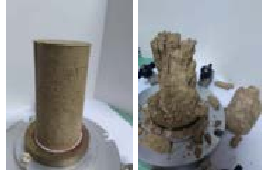
Figure 4 Compressive strength of treated samples before and after testing, series of 28 days old.
