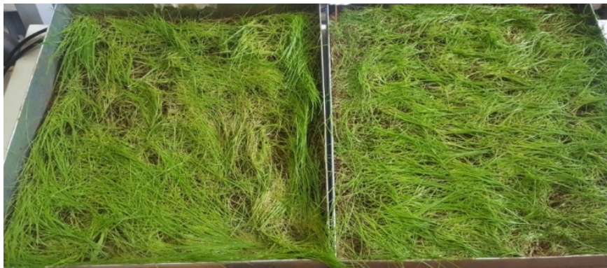
Figure 8 Erosive changes of slopes with vegetation, polymer-improved slope (left side), and natural slope (right side)
