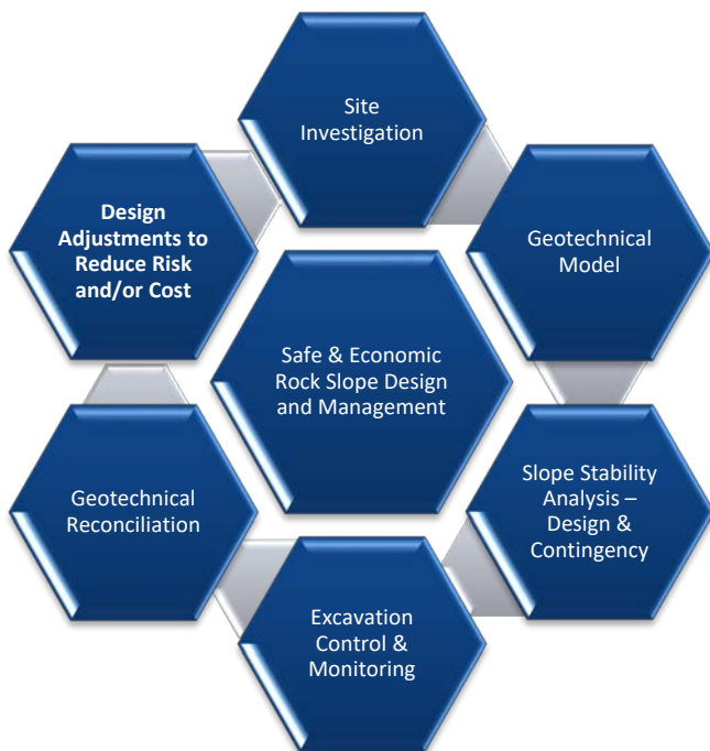
Figure 4 Continuous Improvement Framework for Safe and Economic Rock Slope Design and Management
