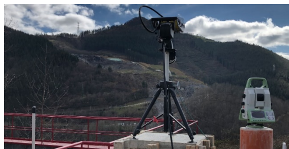
Fig.4. Combination setup radar technology and geodetic technology
