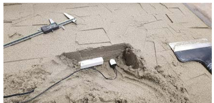
Figure 3 Detail of the installation of the soil moisture sensor and the mini-tensiometer at the monitored point I 1 -6.
