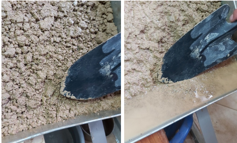
Figure 7 Eroded soil in 180 minutes of rainfall for polymer-improved slope (left side) and natural slope (right side).
