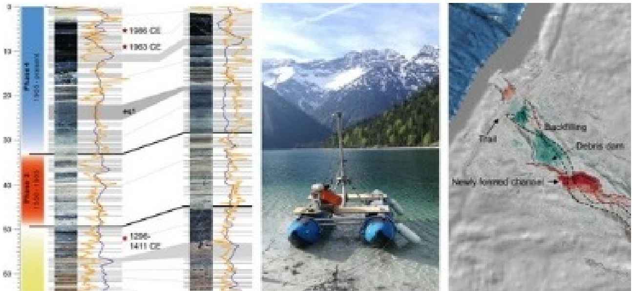
Fig. 4: Debris flow layers in a short core from the Plansee (left), the drill rig (mid) and lake bathymetry showing underwater debris flow deposits (right).
