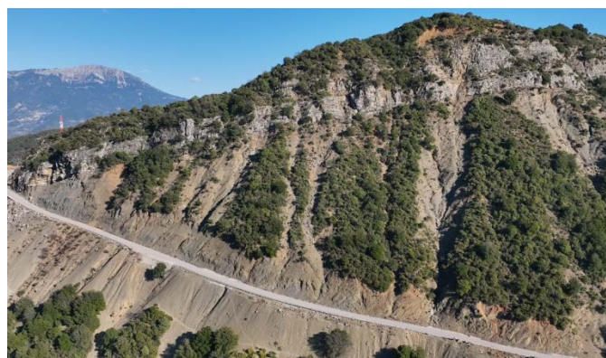
Figure 2 Aerial view of the Valaora region illustrating steep terrain where rockfalls threaten the road and public safety. Visible scars across the landscape mark recent rockfall events, underlining the need for continuous monitoring and mitigation. The potential trajectories of rockfalls from the upper sections of the slope, through thalwegs, to the road level are of particular concern.
